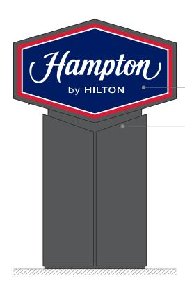
4 mm opal acrylic applied with: 3M 3630-8722 blue vinyl laminated to 3635-20B white blackout, outer border 3M 3630-53 red, outer stripe 3M 3635-20B white blackout
